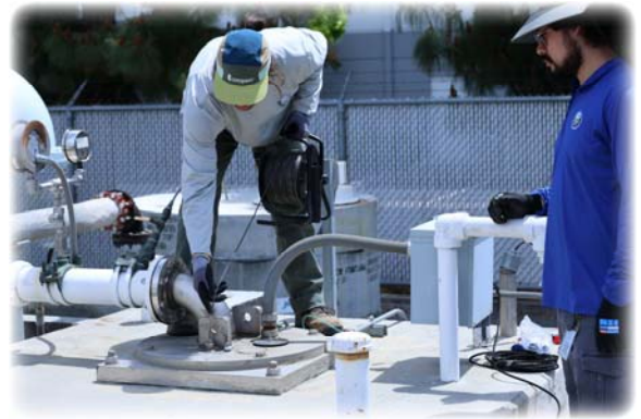
Watermaster Staff Taking Groundwater Level Measurement
